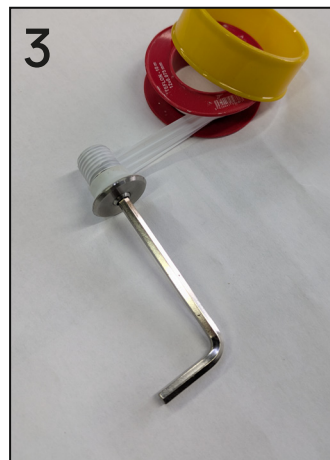
munirsi di: _ chiave a brugola 4mm _ nastro Teflon equip yourself with: _ Allen key - 4mm hexagonal _ Teflon tape
