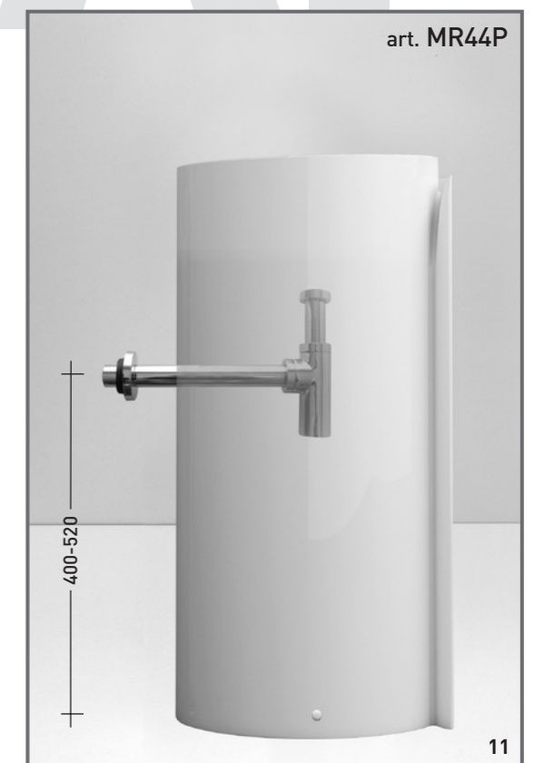
11 Monoroll 44 parete, art. MR44P: per il collegamento dello scarico a parete usare un sifone a bottiglia come illustrato. Monoroll 44 wall column-basin, art. MR44P: connect the basin to the water outlet using a siphon as shown.
